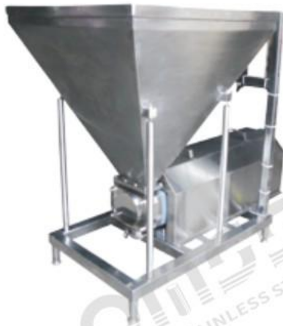
Stuffing product feeding rotor pump(top in,bottom out)
